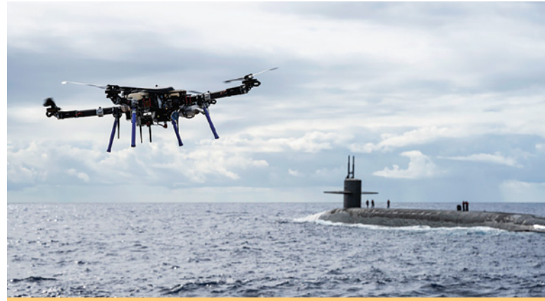
A drone leaves a ballistic missile submarine after delivering a replenishment package. U.S. NAVY
