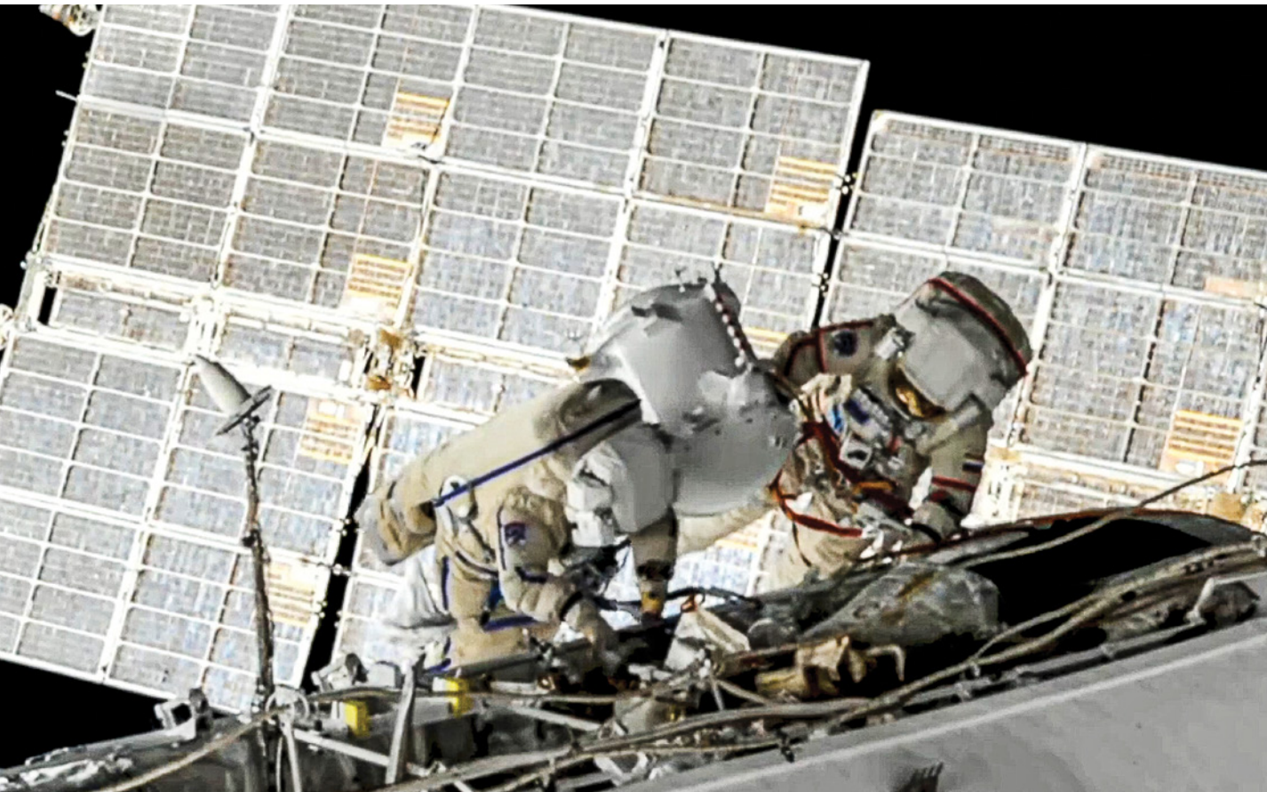
Russian cosmonauts replace old batteries on the International Space Station in June 2021.
