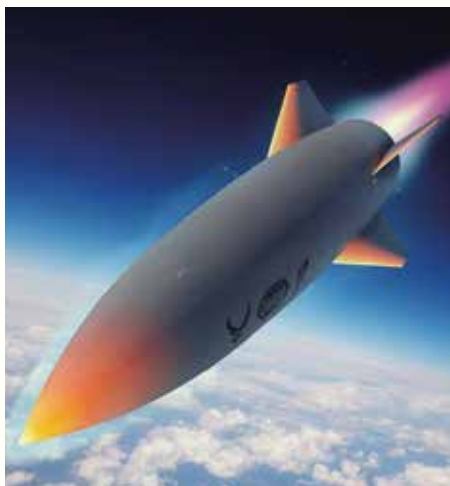
The HAWC vehicle reached an altitude higher than 65,000 ft at a Mach 5 speed and travelled over 556 kilometres
