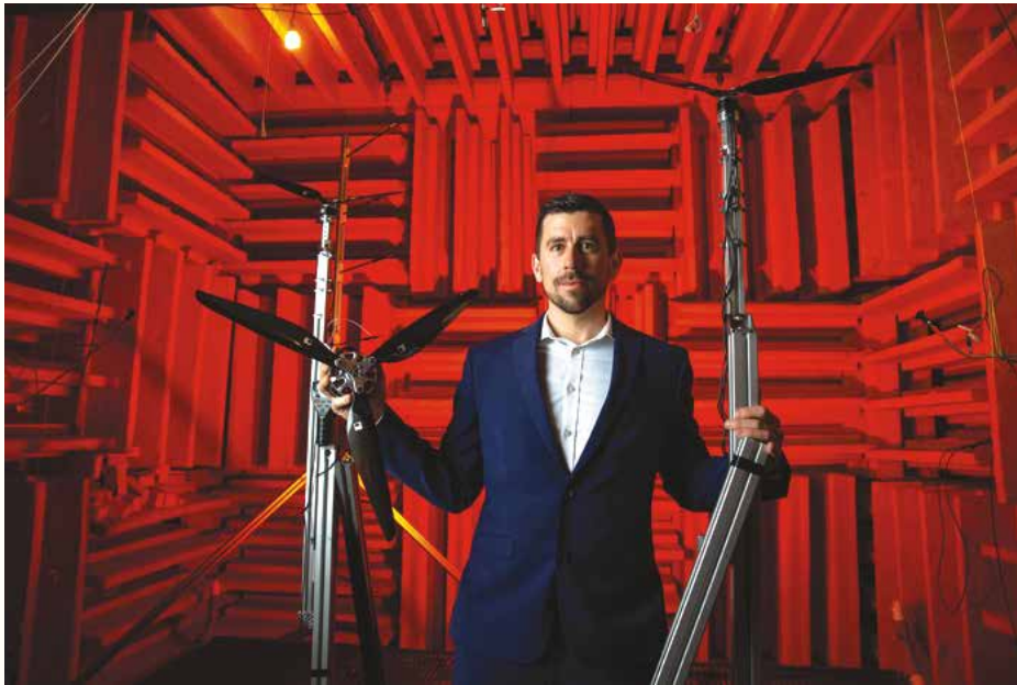
UC aerospace engineering professor Daniel Cuppoletti uses an anechoic chamber covered in sound-absorbing panels to study engine and propeller noise in drones and flying cars
