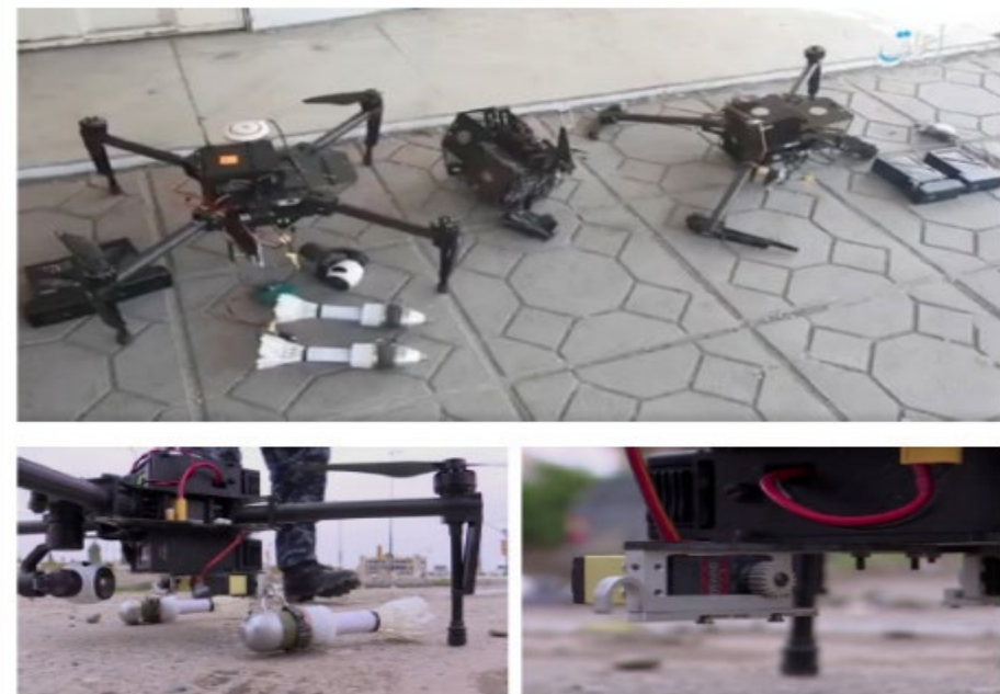
IMAGE 6. MUNITION-LOADED FOUR-PROPELLER DRONE
